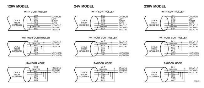
Figure 3. Wiring Diagrams - 120V, 24V and 230V Models
